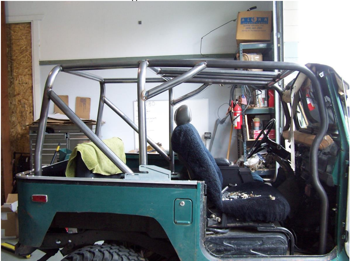
10. If you have handles, dash cross bars, hip guards, rear seat belt bar install at this time.
