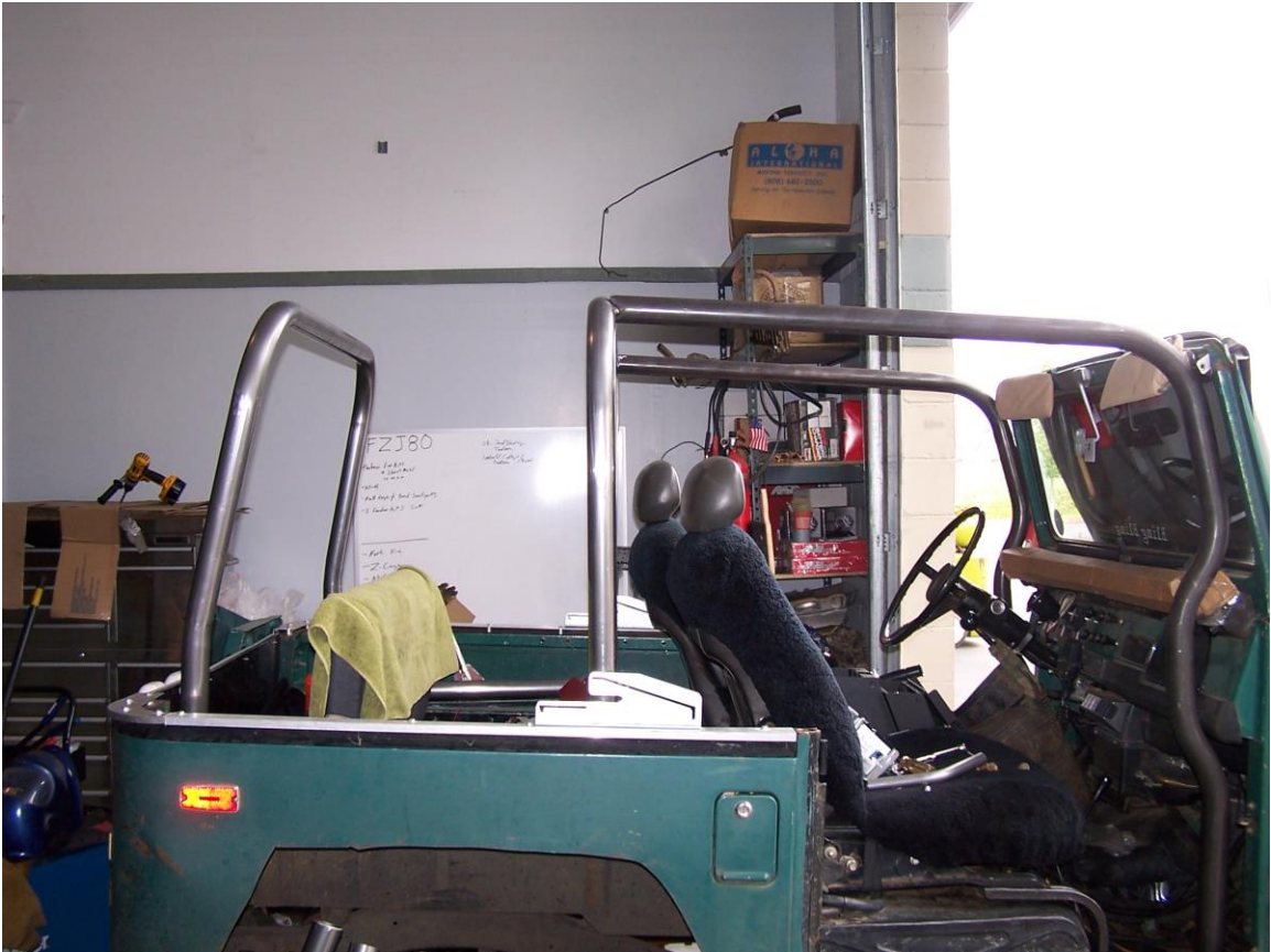
5. Notch and tack the Profile A pillars in place
