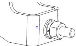
6.3 The remaining threads of the two bolts are the mounting studs for the Hi-lift to hang from. The end of the jack with the mechanism goes to the right of the truck. Use the two remaining nuts to secure the jack to the studs.
