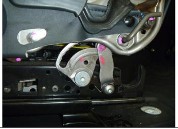
7. Once all the hardware has been removed you can now start to assemble the Metal Tech FJ Cruiser Seat Bracket system onto the FJ Cruiser slider tracks. First you will want to pre-assemble the front and rear mounts loosely with the 3/8" carriage bolts. You will have the carriage bolt on top with a flat washer, lock washer and nut on the bottom
