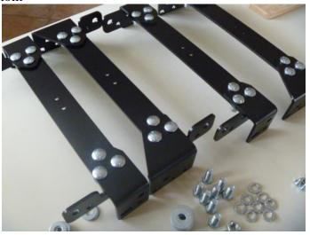
8. Next assemble the mounting plates onto the FJ Cruiser slider track system loosely. You will be using the 5/16" bolts for the front mounting plates and the factory hardware for the rear mounting plates. For the passenger side mount the vehicle occupancy sensor tab using the small ½" bolts to the front of the mounting bracket as shown in the picture below.
