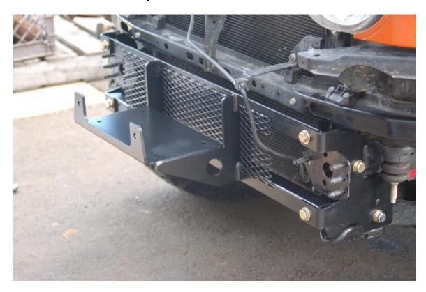
Follow you winch manufactures instructions and install your winch now. The control solenoid box will mount on the supplied bracket to the bumper, so mount this last. You can also mount the controller box under the hood as well.
