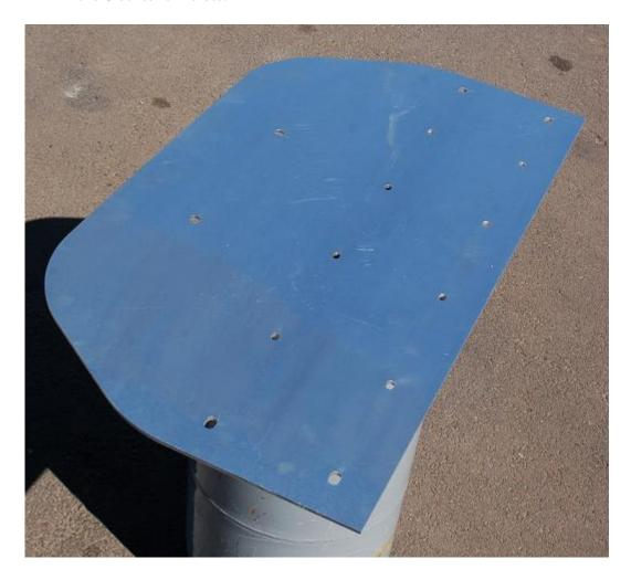
2. Set the back side support on the main bash plate. Make sure the bent edge that is 90\* is facing up and the 30\* edge is facing down over the edge of the back plate. See photo:
