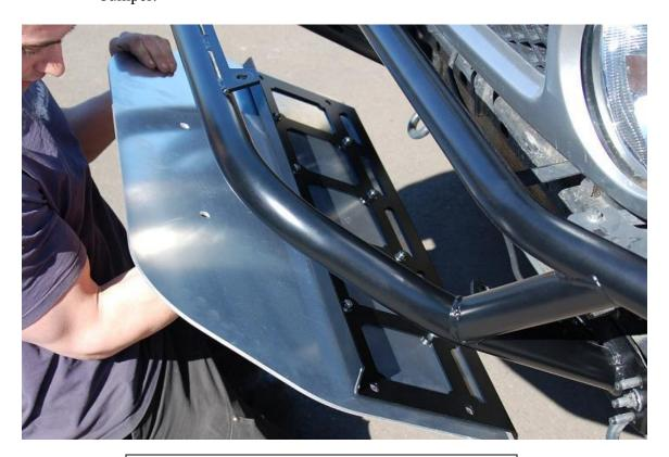
7. Using the provided four 3/8" x 2.5" stainless steel button head bolts, eight washers and four nylock nuts, bolt the bash plate in place with the provided tube spacer between the bash plat mid brace and the inner face of the mounting tabs on the tube bumper.
