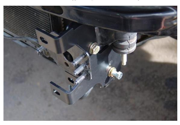
10. **[TOOL:** 34" socket, 34" box end wrench] Install a ½" washer and ½" lock washer inside the frame on the ½" bolt you just installed. Tip: To hold and thread the ½" nut using the 34" box end wrench, put a small piece of packing tape over one side of the box end wrench. See photo:
