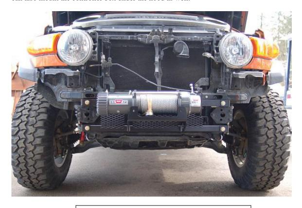
19. Before you install the bumper the lower bracket below the factory head lights either need to be trimmed or removed. We recommend trimming them as they help support the paint matched trim piece below the turn signal as well as the head lights them selves. (Tip: You may want to continue to step 20 but only use one nut per side to hold the bumper on. Then you can fit your lights and easily pull the bumper off to make any modifications needed.) See photo:
