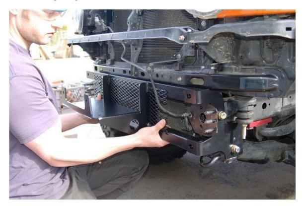
14. **[TOOL: 17mm socket, ¾" socket, ¾" box end wrench]** Install the passenger side, winch side plate. Once the plate is on the side of the frame the ½" dowel pin will hold the plate in place. Install winch mount lower ½" x 3" bolt to hold the winch beam in place. See photo:
