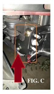
3.5. **[TOOL: 3/4" socket, 3/4" box end wrench]** Install a 1/2" washer and nut on the bolt you just installed. Tip: To hold and thread the 1/2" nut using the 3/4" box end wrench, put a small piece of packing tape over one side of the box end wrench and fold over to trap the nut inside. (Fig D) It is best if you loosely assemble the bracket for now.
