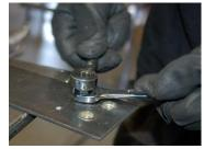
**Pictured Above:** Tool being used it install rivet nut (wrench on nut and wrench on bolt (in house we use an electric impact driver for a quick and easy install)
