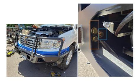
18.0 Work backwards from Step 3 to reinstall wheel well lining (trim accordingly as needed), Grill Fasteners, and any electrical connections.
