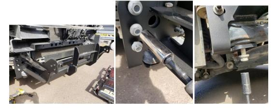
12.0 Insert the 19mm support rod into hole and grab the wedge connector you placed in the side earlier (step 10.0)
