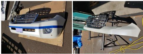
14.0 Install grille back onto your truck and cover the front with painter's tape or similar to prevent scratches when installing the bumper shell.
