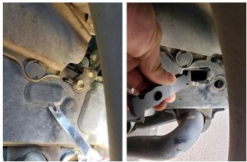
11.0 Set Winch Mount on front of vehicle and attach with original 14mm nuts on the vertical surface and 17mm on the bottom. Do not fully tighten yet as you may need to move the winch mount side to side for alignment purposes later.
